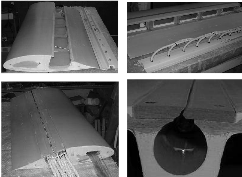
Fig. 13 Building of the model: a) wing building, open model; b) wing building, tubing connection; c) final model; and d) slot.
